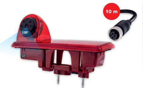
Sensor: 1/3" CMOS Resolution: 800 TV lines Field of view: 120° 10 x LED: backlight dusk/night Night vision distance: 10.66 m **Resolution:** 762 (H) × 504 (V) Power supply: 12/24 V Min. illumination: 0.01 Lux Operating temperature: -20°C-70°C Waterproofing: IP68
