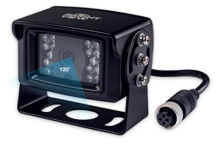
Sensor: 1/4" Sony CCD Resolution: 700 TV lines Field of view: 120° 18 x LED: backlight dusk/night Night vision distance: 7.62 m Resolution: N: 510 × 492 pixels, P: 500 x 582 pixels Power supply: 12/24V Min. illumination: 0 Lux Operating temperature: -10 °C - 65 °C Waterproofing: IP68
