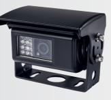
Sensor: 1/3" CCD Resolution: 420 TV lines Field of view: 130° 12 x LED: backlight dusk/night Night vision distance: 7.62 m Resolution: N: 510 × 492 pixels, P: 500 × 582 pixels Power supply: 12/24 V Min. illumination: 0.1 Lux
