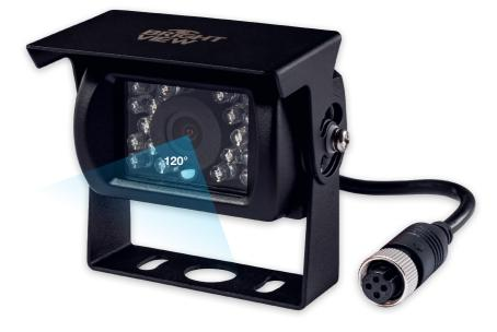
Sensor: 222 SONY/CMOS Resolution: 600 TV lines Field of view: 120° 10 x LED: backlight dusk/night Night vision distance: 7.62 m **Resolution:** 1280 (H) × 960 (V)/ 1280 (H) × 960 (V) Power supply: 12/24 V Min. illumination: 0.1 Lux
