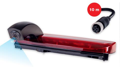
Sensor: 1/3" CMOS Resolution: 800 TV lines Field of view: 120° 8 x LED: backlight dusk/night Night vision distance: 10.66 m **Resolution:** 762 (H) × 504 (V) Power supply: 12/24 V Min. illumination: 0.01 Lux Operating temperature: -20°C-70°C
