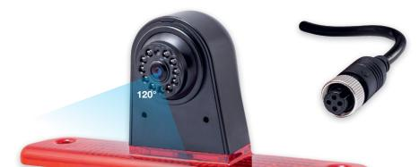
Sensor: 1/3" CMOS Resolution: 800 TV lines Field of view: 120° 10 x LED: backlight dusk/night Night vision distance: 10.66 m **Resolution:** 762 (H) × 504 (V) Power supply: 12/24 V Min. illumination: 0.01 Lux Operating temperature: -20°C-70°C
