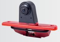
Sensor: 1/3" CMOS Resolution: 800 TV lines Field of view: 120° 10 x LED: backlight dusk/night Night vision distance: 10.66 m **Resolution:** 762 (H) × 504 (V) Power supply: 12/24 V Min. illumination: 0.01 Lux Operating temperature: -20 °C -70 °C Waterproofing: IP68 **Lens:** 2.9 mm Microphone: no
