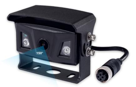
Sensor: 1/3" CMOS Resolution: 700 TV lines Field of view: 150° 2 x LED: backlight dusk/night Night vision distance: 10.66 m **Resolution:** 976 (H) × 592 (V) Power supply: 12/24 V Min. illumination: 0.1 Lux Operating temperature: -20°C-70°C Waterproofing: IP68 Lens: 1.98 mm
