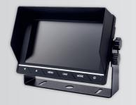
Monitor: 7" LCD Aspect ratio: 16:9 Video output: 2 × 4 pin cable Option: PAL&NTSC, AUTO system Resolution: 800 × 480 RGB Power supply: 12/24 V Consumption: ≥8.64 W **Operating temperature:** -10 °C -65 °C Buttons: touch
