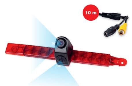
Resolution: 800 TV lines Field of view: 70°/130° **Resolution:** 762 (H) × 504 (V) Power supply: 12/24 V Min. illumination: 0.01 Lux
