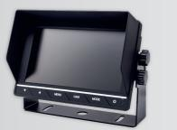
Monitor: 7" LCD Aspect ratio: 16:9 Video output: 2 × 4 pin cable Option: PAL&NTSC, AUTO system Resolution: 800 × 480 RGB Power supply: 12/24 V Consumption: ≥8.64 W **Operating temperature:** -10 °C -65 °C Buttons: touch
