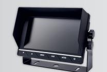
Monitor: 7" LCD Aspect ratio: 16:9 Video output: 2 × 4 pin cable Option: PAL&NTSC, AUTO system Resolution: 800 × 480 RGB Power supply: 12/24 V Consumption: ≥8.64 W Operating temperature: -10 °C -65 °C Buttons: touch Automatic switch-on when reversing Automatic brightness adjustment according to outside light
