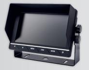
Monitor: 7" LCD Aspect ratio: 16:9 Video output: 2 × 4 pin cable Option: PAL&NTSC, AUTO system Resolution: 800 × 480 RGB Power supply: 12/24 V **Consumption:** ≥8.64 W **Operating temperature:** -10 °C -65 °C Buttons: touch Automatic switch-on when reversing Automatic brightness adjustment according to outside light Menu: EN, DE, FR, ES, PT, IT
