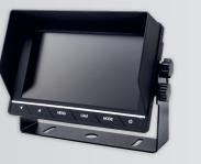
Monitor: 7" LCD Aspect ratio: 16:9 Video output: 2 × 4 pin cable Option: PAL&NTSC, AUTO system Resolution: 800 × 480 RGB Power supply: 12/24 V Consumption: ≥8.64 W **Operating temperature:** -10 °C -65 °C Buttons: touch Automatic switch-on when reversing
